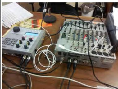
Our new Outdoor Broadcast set-up, with the Codec on the left and mixer on the right
